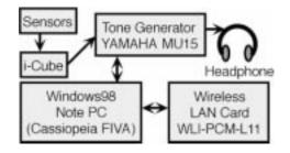
Fig. 10 Construction of prototype CosTune.
