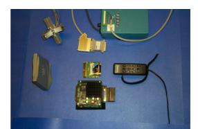
Figure 4. Components of the inertial tracker. The cross-shaped device in the upper left is the inertial tracker. The microprocessor (lower center) is worn by the user, and broadcasts tracking data offboard to the base station (lower left).
