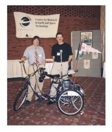
Figure 1: The Virtual Reality Tricycle. The VR Trike permits different combinations of visual and non-visual cues to be presented to an operator, but uses a HMD to generate the visual cues.
