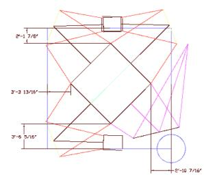
(a) Autocad drawing showing layout of the four vertical walls, the projectors (mounted in two stacks at the top and bottom of the image), and the four featherlight mirrors.
