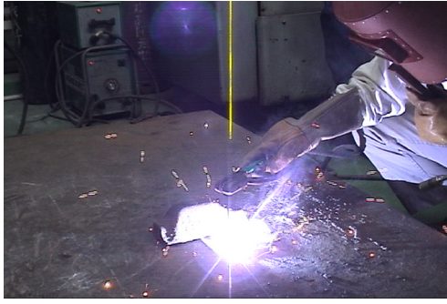
Fig. 1: A scene of manual metal arc welding. The welder put on the face shield and thick hand glove. Strong visible rays and ultraviolet rays were radiated during welding.
