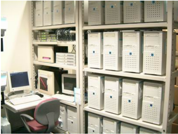
Fig. 8 PC cluster for parallel processing
