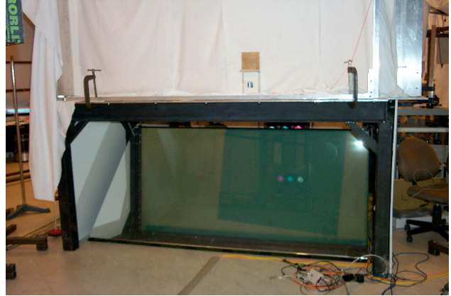
Figure 4. Details of the ceiling (left) and floor (right). The ceiling is suspended from the ceiling of the laboratory on cables that permits the ceiling to be raised slightly above the walls to provide better air flow, and lowered (when the walls are removed) to permit servicing. The mirrors are mounted on adjustable rods to permit adjustment of the projection angle. The floor mirror is mounted to the floor support. You can see the projector reflected in the floor mirror. On the right hand side of the ceiling mirror you can see the vertically placed projector.
