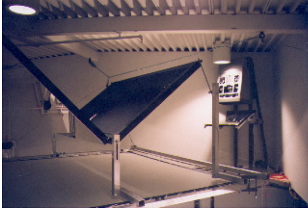
Figure 4. Details of the ceiling (left) and floor (right). The ceiling is suspended from the ceiling of the laboratory on cables that permits the ceiling to be raised slightly above the walls to provide better air flow, and lowered (when the walls are removed) to permit servicing. The mirrors are mounted on adjustable rods to permit adjustment of the projection angle. The floor mirror is mounted to the floor support. You can see the projector reflected in the floor mirror. On the right hand side of the ceiling mirror you can see the vertically placed projector.
