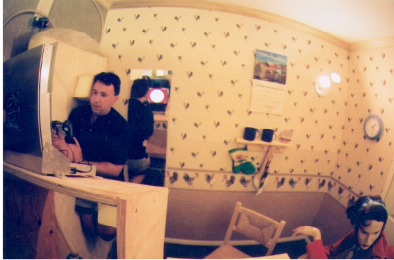
Figure 1. The Tumbling and Tilted Room. (a) The Tumbling room is an 8' cube mounted on a horizontal axis. The room can be rotated about this axis under computer control. (b) The Tilted room is an 8' cube built rotated by 90 degrees. The left panel shows what the subject sees (the subject is actually lying right side down on the floor), the right panel shows the true situation.
