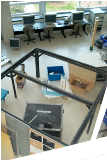
Figure 2. View of the floor support taken from the 2 nd story of the VGR lab. A catwalk around the space provides access to the projectors and mirrors. Note that IVY's floor is located 4' above the physical floor of the lab.
