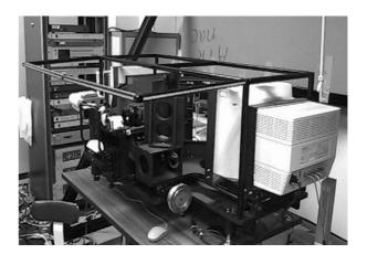
Fig. 3 Stereoscopic display with the accommodative compensation (3DDAC)
