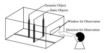
Fig. 4 Inspection method of the visual acuity for the depth
