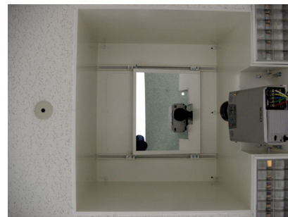
Fig. 4: The camera and the projector (using a mirror because the ceiling is not high enough)
