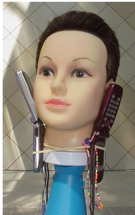
Fig. 7: “Poor person’s mobile stereotelephony:” two mobile phones deployed as a microphone array attached to a dummy head simultaneously calling a dual voice line (like that provided by ISDN) realizes wireless (if still low-fidelity) binaural telepresence.
