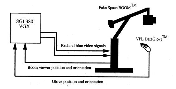
Figure 6: The system configuration of the virtual windtunnel
