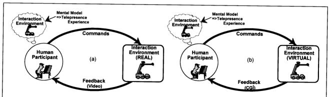
Fig. 1 Generic representation of telepresence: a) Telerobotics: Human participant experiences interaction of remote manipulator with real environmental objects; b) Artificial Reality: Human participant experiences interaction with computer simulation of both manipulator and environmental objects.
