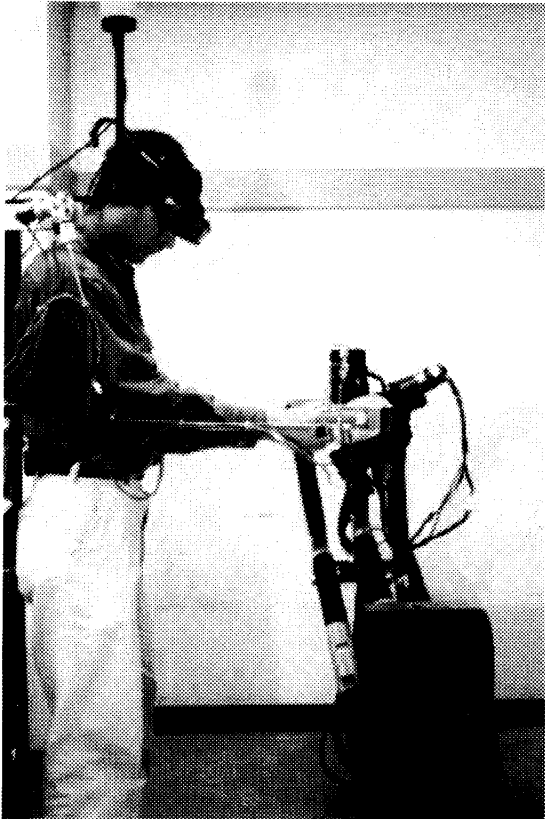
Fig. 2 General View of the Haptic Graphic Device which Generates Shape of a Virtual Object
