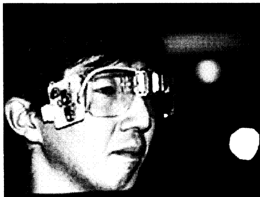
Fig.7 Ultrasonic eye glasses for the blind
