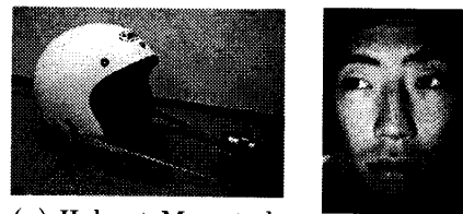
(a) Helmet Mounted Camera (b) Video Image Figure 14: Helmet Mounted Camera and Video Image
