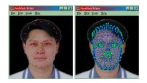
Figure 9. The wireframe model resulted from feature point selection.
