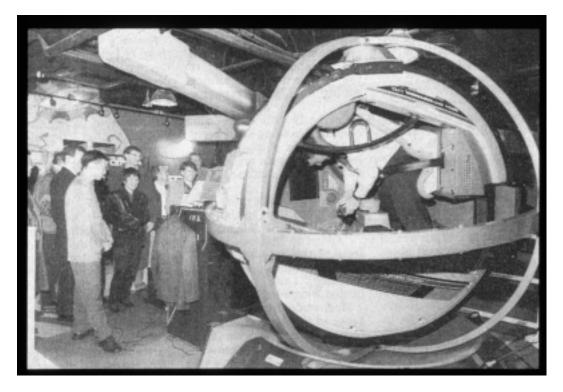
Fig. 3: R360 (SEGA): jet fighter simulator with gimbals providing three rotational degrees of freedom
