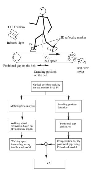
Figure 2: Block diagram of the control mechanism in the ATLAS
