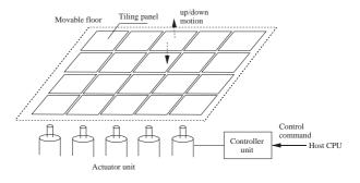
Figure 3: Basic concept of the ALF system
