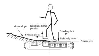
Figure 6: Schematic of the virtual slope
