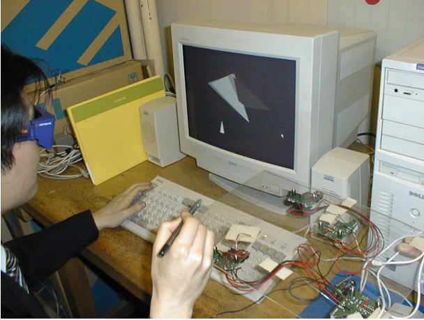
Fig. 4 3-sensors version 3-D Mouse
