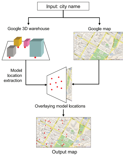
Figure 4: Map production flow. First, a city name is queried. The tool extracts the map and 3D models of the city. The local database for initialization are then built. The 3D model positions are overlaid as the colored dots.
