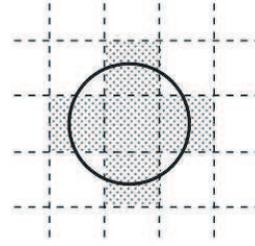
Figure 3: Agent Behavior Decision Model. The circle shows agent's body, and the cells occupied by only one agent. The agent selects its own direction of movement from five cells (forward, back, left, right, stay here). These cells are smaller than the agents' scale. Then, the agent moves with no constraint except that if the target cell is closed or is a wall.
