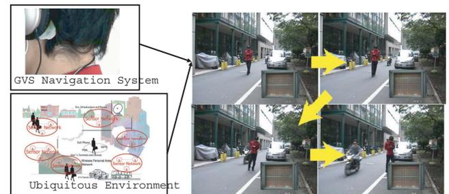
Figure 1: Human Behavior Induction by GVS. By using GVS and the environmental information provided by sensor networks, the wearer of PH can avoid a motorcycle, unconsciously
