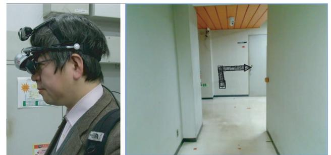
Figure 2: Prototype Wearable Navigation System using AR Technology. Left: The rapid prototype of the HMD of the PH. Right: The image for the wearer of the PH.
