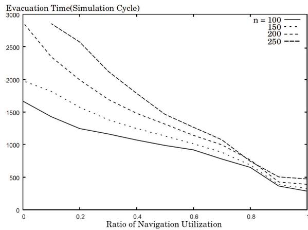
Figure 12: The average time of evacuation. Each line is different density of agents  $N = \{100, 150, 200, 250\}$ . The x-axis is the ratio of navigation utilization. When all pedestrians are provided the support from navigation system, the average time of evacuation decreases.
