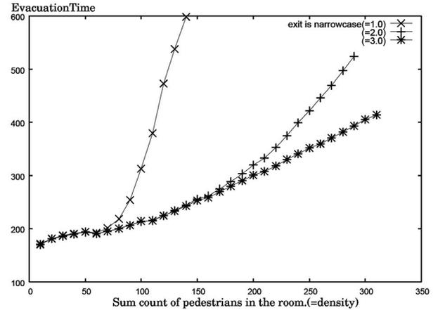
Figure 6: The average time of evacuation depending on entrance width: There are entrances, which are two types of width  $W$ . the narrow ( $W = 1.0$ ) and the wide ( $W = 2.0, 3.0$ ). The narrow line increased exponentially earlier than the wide line.
