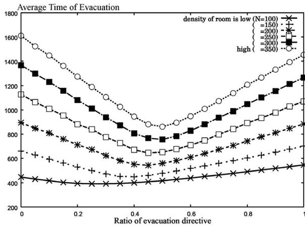
Figure 9: The average time of evacuation: Each line is different density of agents  $N = \{100, 150, 200, 250, 300, 350\}$ . The x-axis is the ratio of pedestrians  $\alpha$ , who leave via Exit B. The y-axis is the average time of evacuation of all pedestrians. When  $\alpha$  is around 0.5, all pedestrians escape efficiently.
