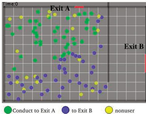
Figure 7: Simulation Field: Field size is 10m x 15m. This situation has two possible escapes: Exit A and B. Exit A is narrow, but is known by all pedestrians. Exit B is wide, but not all pedestrians may know its existence.
