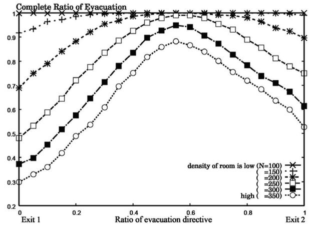
Figure 10: The ratio of escape completion: Each line is different density of agents  $N = \{100, 150, 200, 250, 300, 350\}$ . The x-axis is the ratio of pedestrians  $\alpha$ , who leave via Exit B. The y-axis is the ratio of pedestrians who complete the evacuation by certain counts (= 2000 steps).
