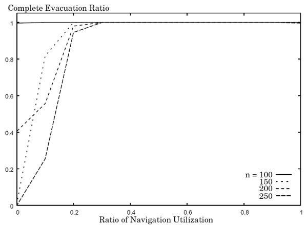
Figure 13: The ratio of complete evacuation. Each line is different density of agents  $N = \{100, 150, 200, 250\}$ . The x-axis is the ratio of navigation utilization. When  $N$  is 100, all pedestrians finish the escape action completely. In Other conditions, when the system utilization is over 30%, all pedestrians may finish escape action completely.
