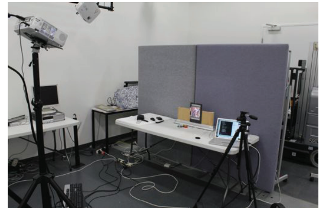
Figure 8: The experimental setup showing a projector on the left mounted at a distance of 2.5-3 metres from the ePaper display.
