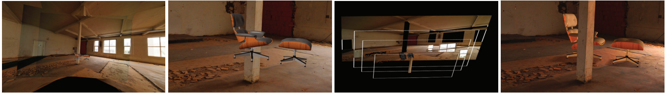
Figure 1: (a) 3D Photo Collection with embedded object, (b) Close-up of unlit object with wrong occlusion. (c) Photo divided into 3D segments (Sliced Image). (d) Convincing augmentation with our occlusion handling and image-based lighting features.
