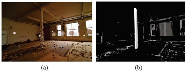
Figure 12: Estimating the depth map: (a) Original image with 3D key points. (b) The corresponding depth map as gray-scale image.
