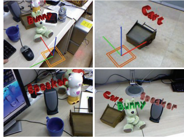
Figure 1: Detection and pose estimation of a 3D object. Our method can detect and estimate the pose of a 3D object. It also provides occlusion between the real and the virtual object based on depth information.
