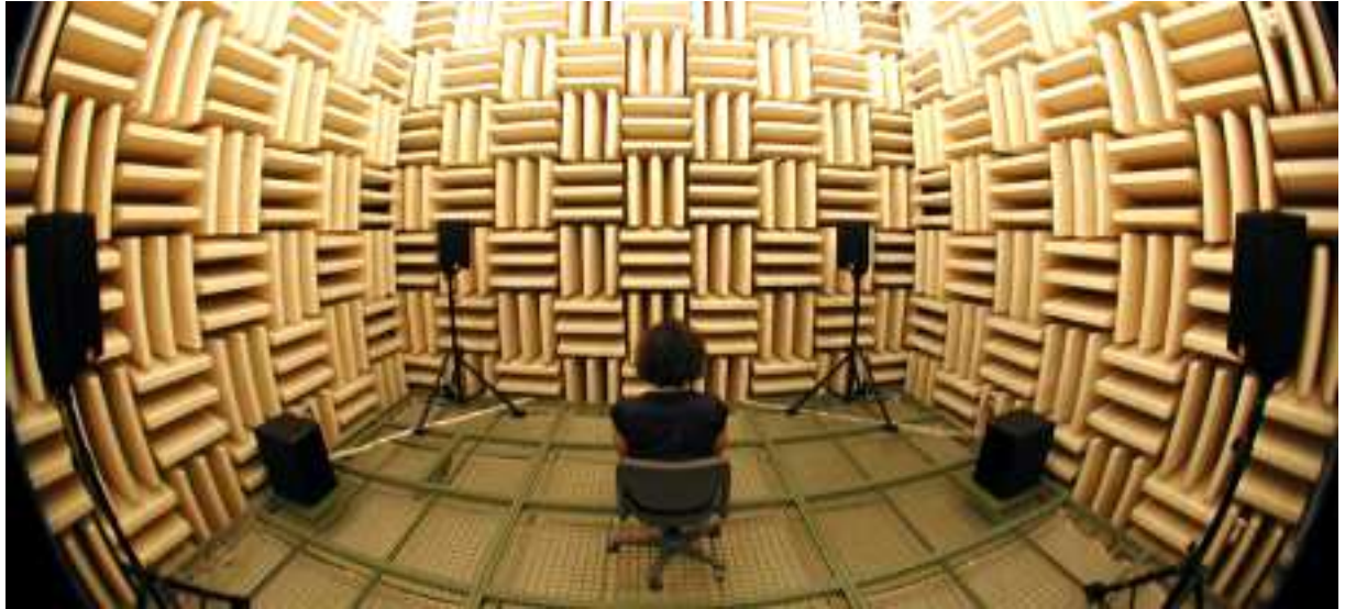
Fig. 2: The 4-channel loudspeaker setup in the University of Aizu’s large anechoic chamber.
