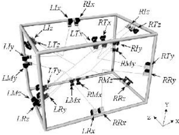
Fig. 2 Location of 24 actuators on the frame
