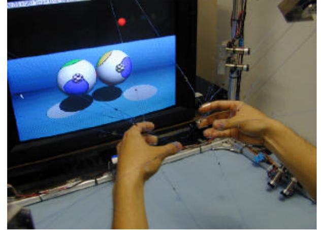
Fig. 7 Fit-The-Face task with virtual spheres using SPIDAR-8
