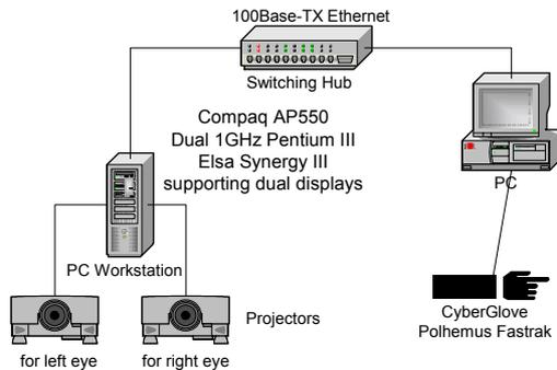
**Figure 19: Hardware configuration of prototype system**
