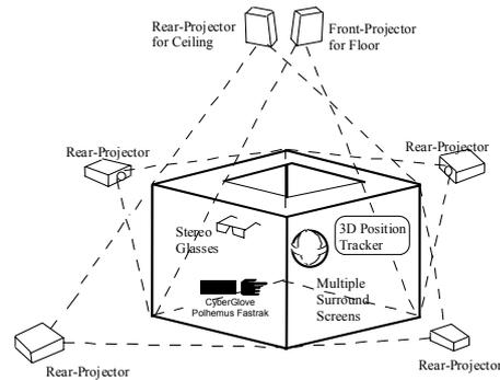
**Figure 20: Schematic diagram of TEELeX**
