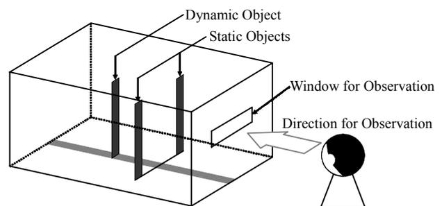
Fig. 4 Inspection method of the visual acuity for the depth
