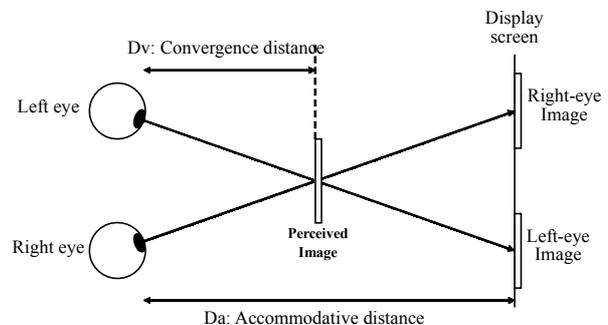
Fig.1 The contradiction between convergence and accommodation in the stereoscopic displays
