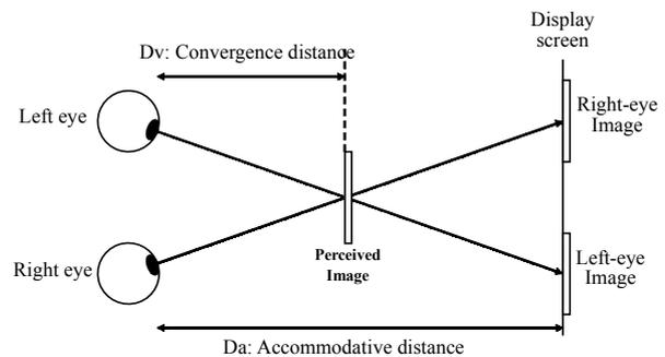
Fig.1 The contradiction between convergence and accommodation in the stereoscopic displays
