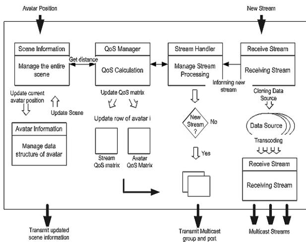
Fig. 5 TIE system architecture for virtual dancing environment
