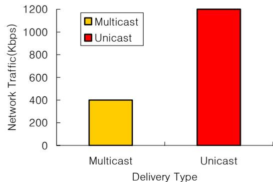
Fig. 9 Packet transmission on the network
