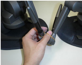
Fig. 5: Pinching manipulation via two PHANTOM Desktops. Two fingers are attached at the joints of the PHANToMs using rubber bands.
