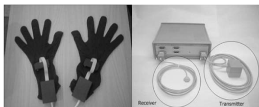
Fig. 8 Data Gloves and Motion Tracking Devices
