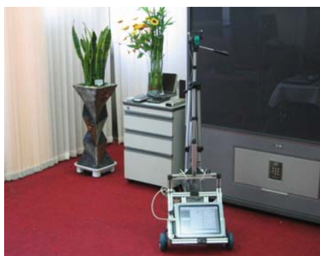
Fig. 6 ER1 robot in the testbed. IR receiver is attached at a height of 120 cm.
