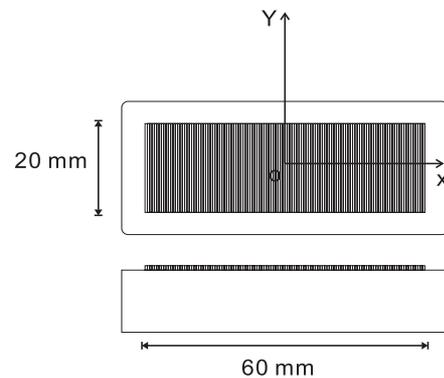
Fig.5 Schematic drawing of the linear array transducer: Top view and side view
