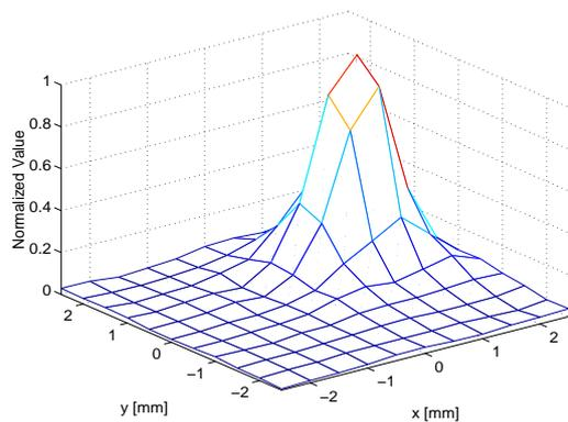
Fig.8 Spatial distribution of acoustic radiation pressure for a single focal point (3D plot)
