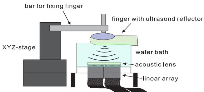
Fig.1 Schematic drawing of the tactile display.
