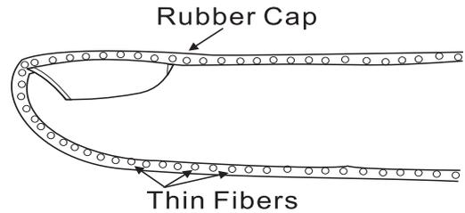
Fig.3 Cross section drawing of the finger cap for reflecting ultrasound
