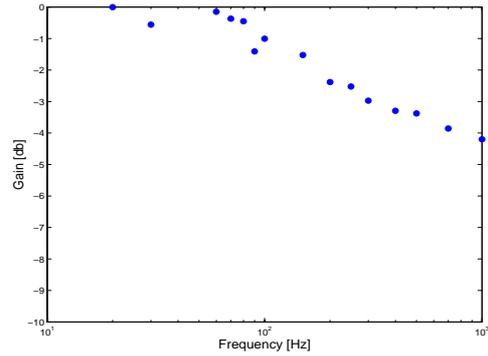
Fig.7 Gain-frequency characteristics of acoustic radiation pressure: Horizontal axis represents frequency of modulated radiation pressure [Hz]. Vertical axis represents dB gain
