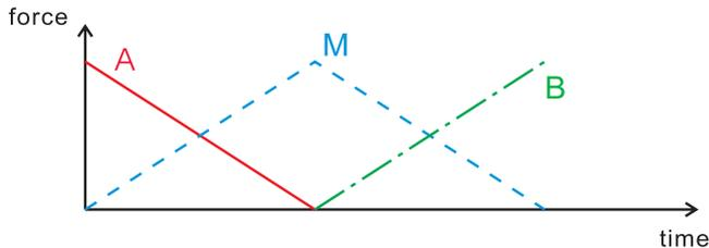
Fig.11 Schematic drawing of time dependent force at each stimulation point in 3PT type stimulation. The solid, dashed and dash-dot lines represent forces applied to A, M and B, respectively. Note that the total amount of force is always kept at the same value and that the center of the force is moved at the constant velocity
