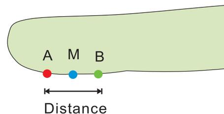
Fig.10 The position of each point on the finger pad. The starting point A is located at the center of the finger pad. The position of the end point B is determined by the parameter “Distance”. M is the midpoint of the line segment AB.
