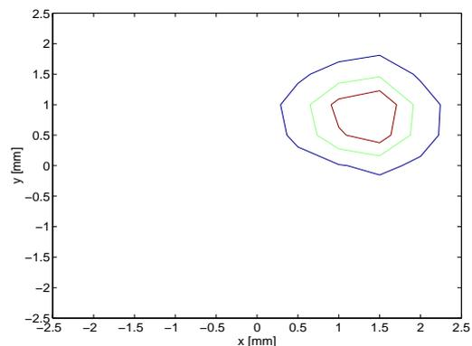
Fig.9 Spatial distribution of acoustic radiation pressure for a single focal point (contour plot): Each line represents 25%, 50%, 75% of the peak value, respectively.
