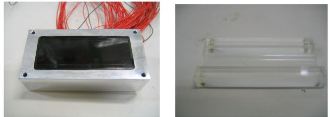
Fig.4 Photograph of the linear array transducer: Left: 120 channel linear array transducer, Right: cylindrical acoustic lens made of acrylic plastic
