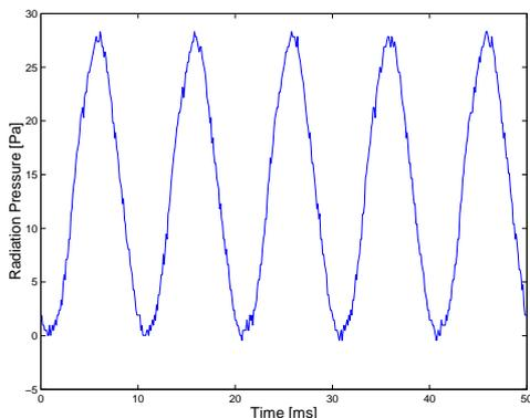
Fig.6 Sinusoidal wave of observed acoustic radiation pressure: Horizontal axis means time [ms]. Vertical axis means the observed acoustic radiation pressure [Pa]
