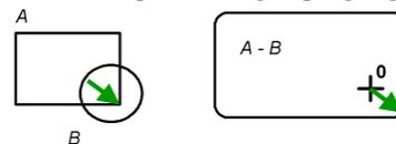
Fig. 4 A pair of intersection objects and their corresponding CSO. The arrow represents the penetration depth
