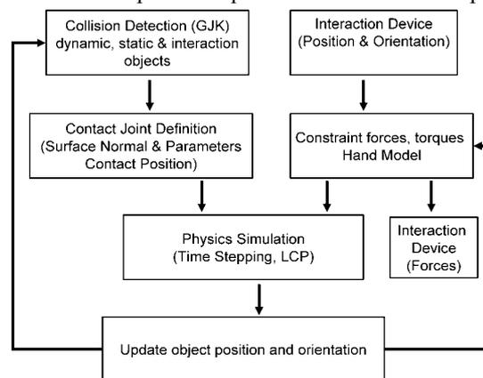
Fig. 3 Simulation sequence of grasping algorithm and
