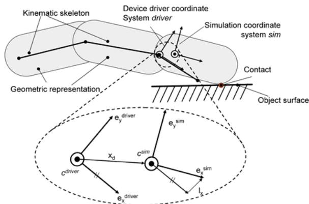
Fig. 1 Schematic view of the implemented constraint mechanism of the hand model
