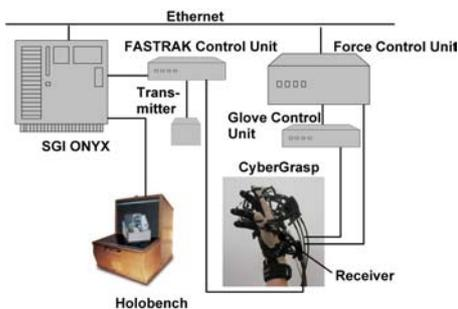
Fig. 5 Hardware setup of  $Ve^2$
