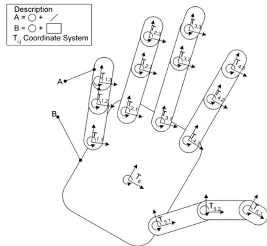
Fig. 2 Approximation of the users hand for the collision detection by the Minkowski sum out of primitives
