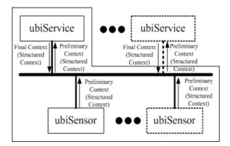
Fig. 2. ubi-UCAM architecture; ubiSensor and ubiService
