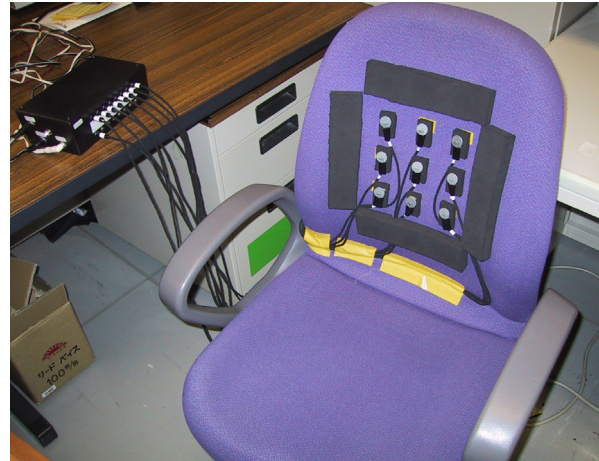
Figure7: Office chair with 3-by-3 tactor array for vibrotactile letter reading tasks
