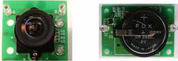
Fig. 3 IR Tracker (left) and IR-LED ID Tag (right)
