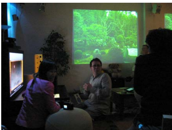
Figure 2 : the Zenetic computer in the sensitive house. The plasma screen is used for main display, while a large rock garden (in front of the author) integrates a sensitive screen for interaction. The yellow box in the back emits smells. Videos are projected on the wall behind. A very dark ambient is used.
