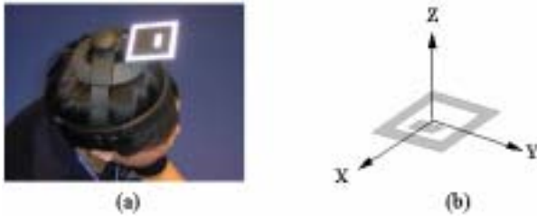
Figure 3. User with the retro-reflective marker (a), and the retro-reflective marker geometry (b).
