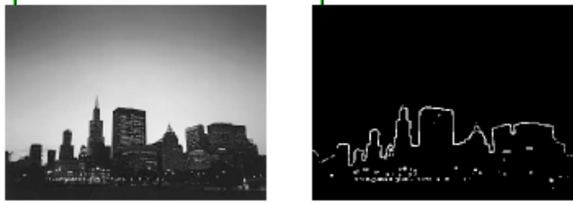
Figure 4. Image before and after applying the Sobel edge detection algorithm.
