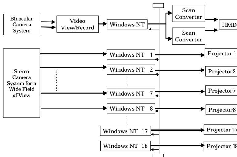
**Fig.11 Architecture of the Augmented Reality System**
