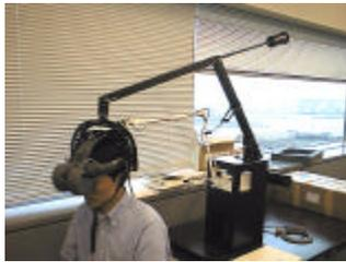
**Fig.7 The Developed HMD System with Head-tracking Function**
