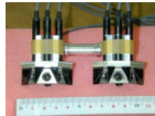
**Fig.5 Photograph of the Developed Stereo-multi-camera System for a Wide Field of View**
