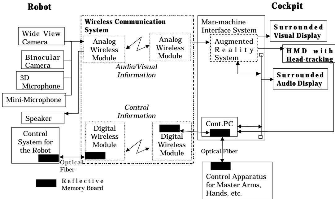
**Fig.10 Total Hardware Architecture of the Man-machine Interface**
