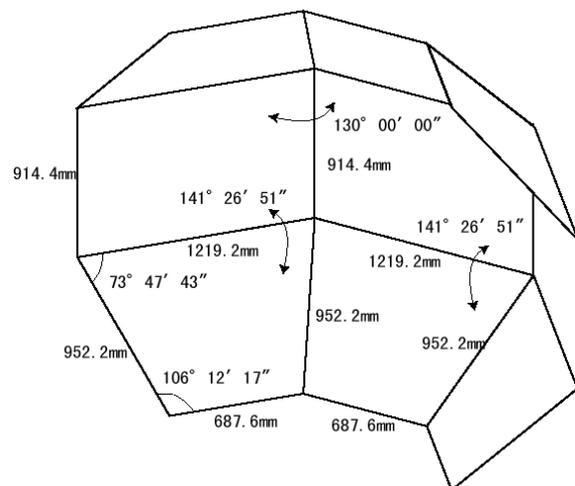
Fig.2 Design Diagram of the Surrounded Visual Display System
