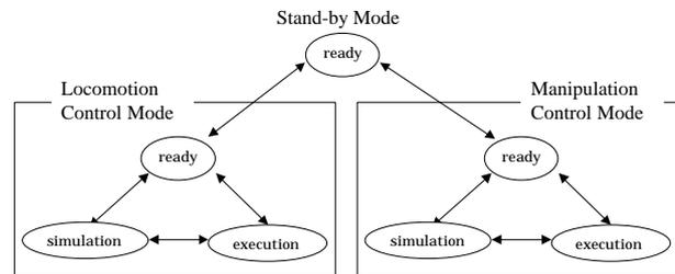
**Fig.9 A State Transition Diagram of a Man-machine Interface**
