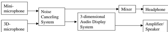
**Fig.8 A Block-diagram of the Stereo Audio Display System**
