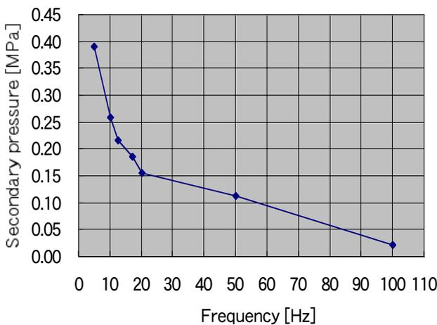
**Fig. 6** Operational frequency vs. Secondary pressure of a control valve
