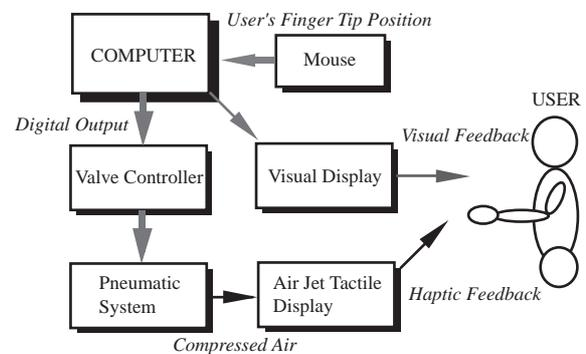
**Fig. 9** System configuration for perceptual characteristics
