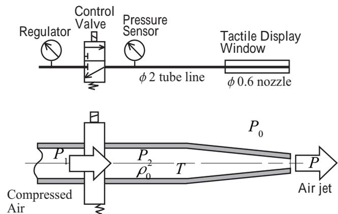
**Fig. 7** one dimensional adiabatic compressible fluid in a convergent nozzle model
