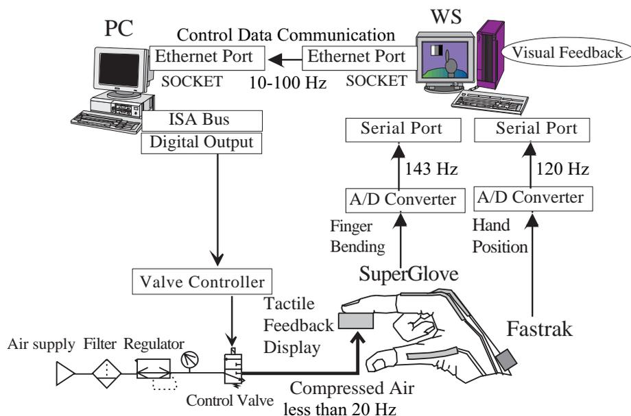
Fig. 15 System configuration for touching in virtual environment.
