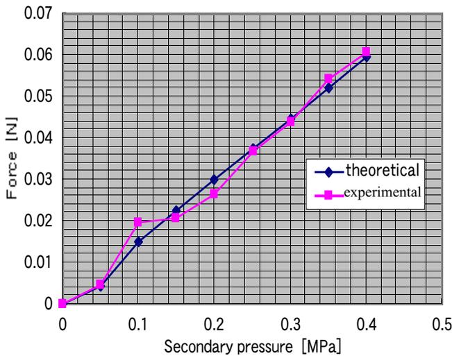
**Fig. 8** Displayed force vs. secondary pressure of control at the outlet surface
