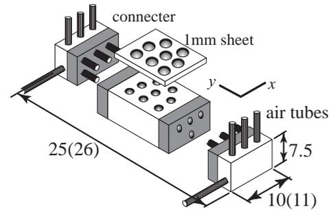
(a) Construction of tactile display
