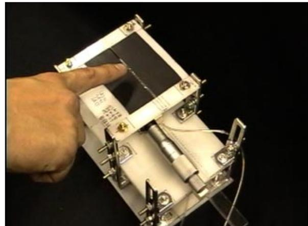
Fig. 2 Apparatus to determine two-point-difference thresholds
