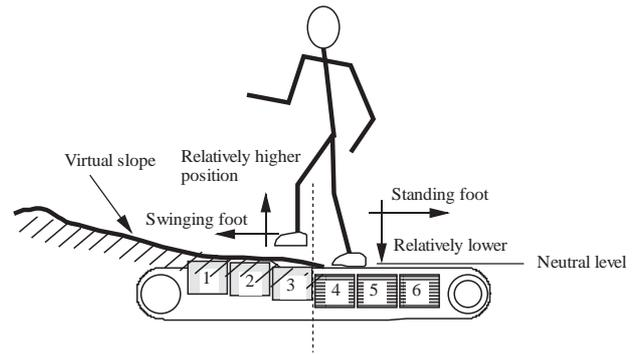
Figure 6: Schematic of the virtual slope
