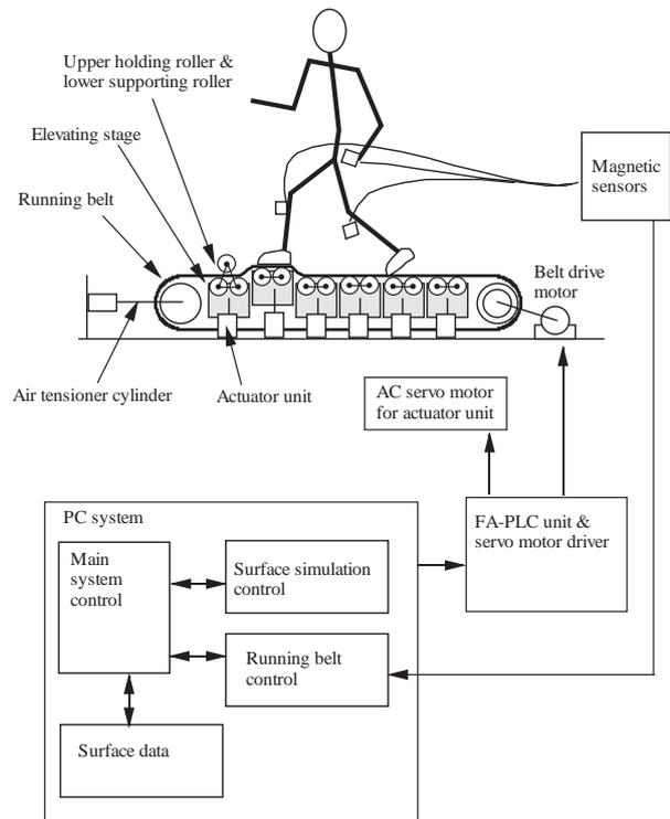
Figure 5: Block diagram of the 1st prototype
