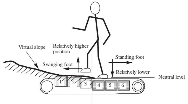
Figure 6: Schematic of the virtual slope
