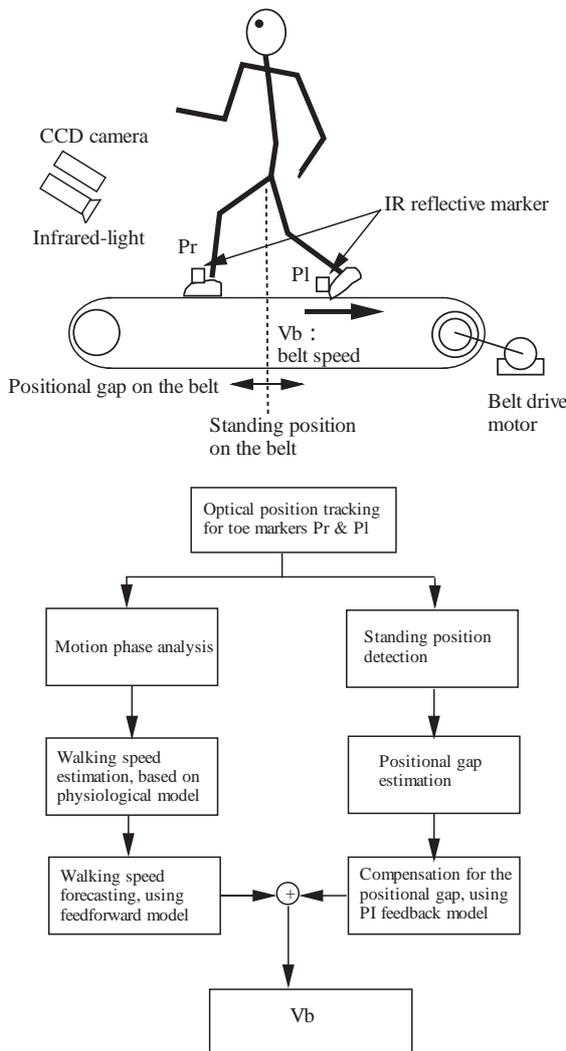
Figure 2: Block diagram of the control mechanism in the ATLAS
