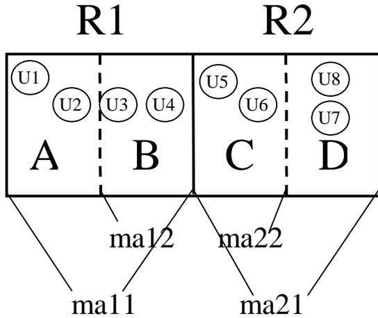
Fig. 3 Assignment of multicast addresses in regions
