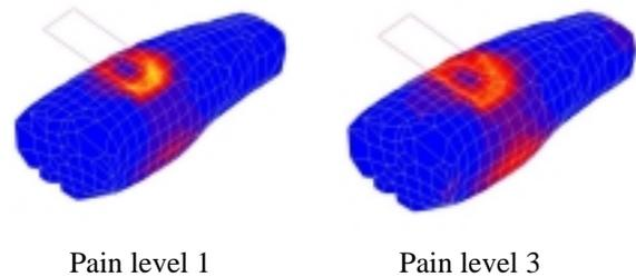
Fig.11 Simulation of contact deformation of forearm by the contact with band-handle of bag and evaluation of the pain level
