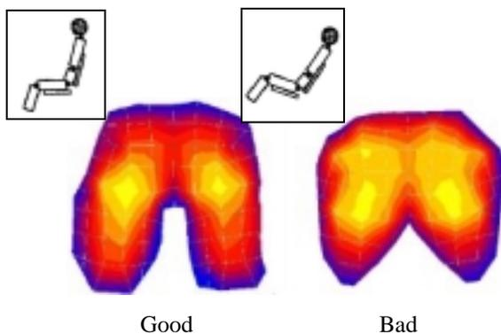
Fig.10 Simulation of contact deformation of buttocks by the contact with chair and evaluation of the comfortability
