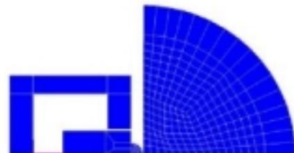
Fig.6 Simulation of hardness testing to obtain relation between hardness and Mooney constant
