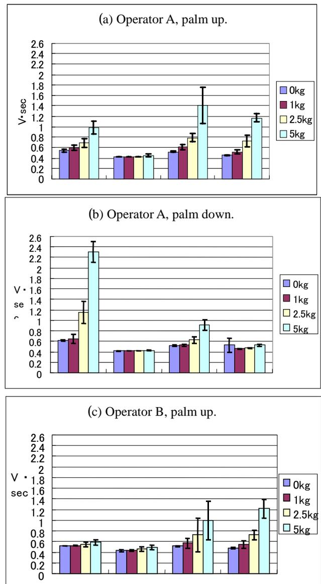
Figure 10: Average of the integral of the EMG signals.
