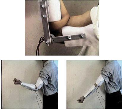
Fig. 2: An elbow joint angle experiment apparatus.
