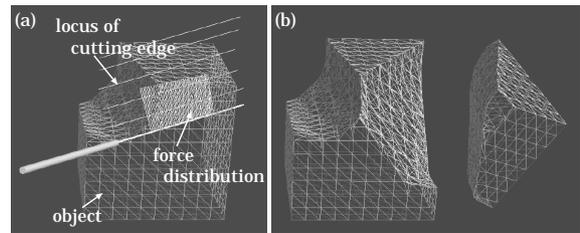
Fig.12: Representation of Cutting Force
