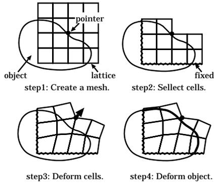
Fig.1: Process of Deforming Operation
