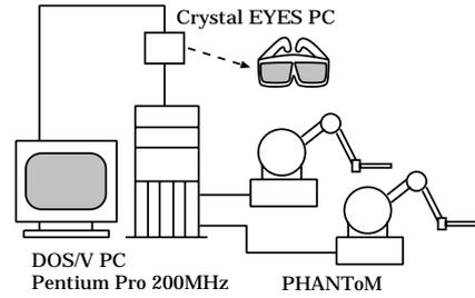
Fig.2: System Construction
