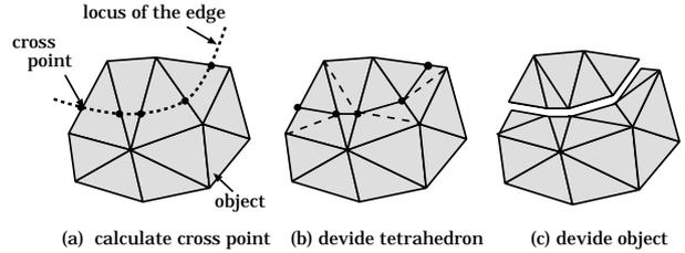
Fig.9: Process of Cutting Operation
