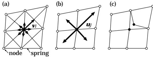
Fig.4: Dividing Spring Model
