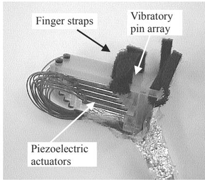
Fig. 1 Texture Display F10. Ten vibratory pins are driven individually by piezoelectric actuators. The F10 is mounted to the index fingertip with finger straps.
