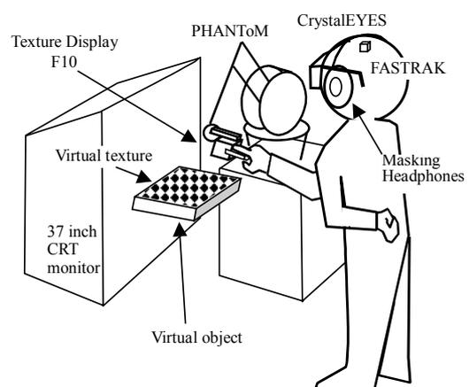
Fig. 7 Texture Display F10++ system setup. The F10 imparts texture information on a virtual object to the user along with force feedback provided by the PHANToM.
