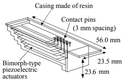
Fig. 2 The frame of Texture Display F10. The frame and contact pins were fabricated of photo-curing resin.
