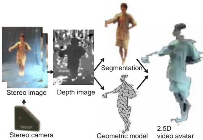
Fig. 5 Basic process of making 2.5 dimensional video avatar
