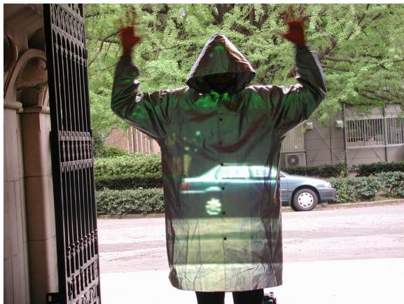
Fig.1 Optical Camouflage using Retro-reflective Projection Technology (RPT).
