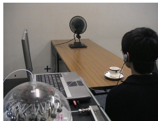
Figure 5: Odor playback with a changing airflow field.
