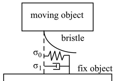
Figure 4. LuGre friction model.
