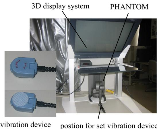
Figure 1. The system is consisted by 3D display and haptic devices.
