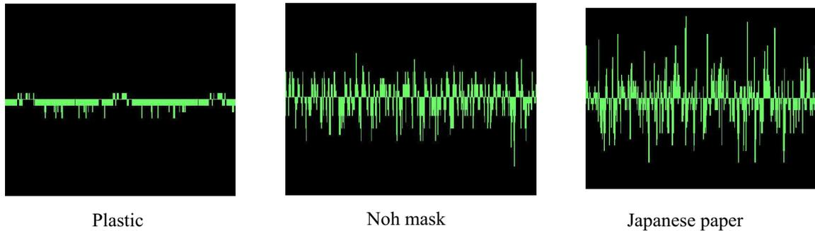
Figure 6. Synthesized vibration signal for tactile device.
